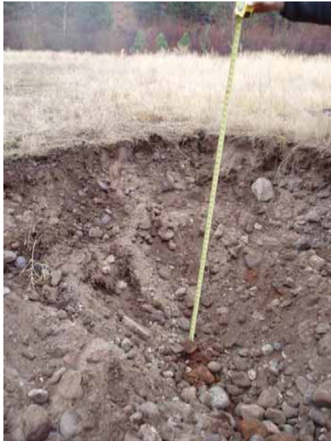
Figure 14. Soil pit in Reach 3. Pit located above Duckett Pond showing the depth and size of relic channel bed.
