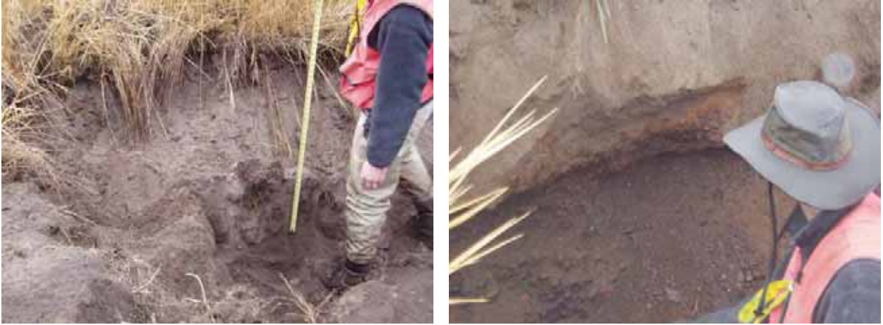
Figure 14. Soil pit in Reach 3. Pit located above Duckett Pond showing the depth and size of relic channel bed.
