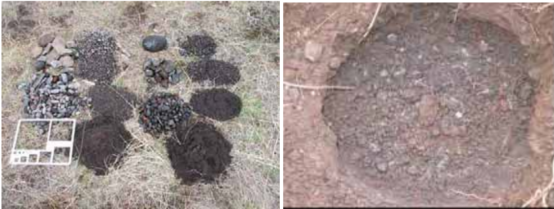
Figure 12. Pavement / sub-pavement samples in the relic channel. Excavating pavement / sub-pavement samples (top), (bottom left) sieved pavement on left, sieved sub-pavement on right, and (bottom right) five inches beneath surface of meadow.
